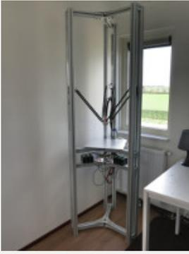
Stefan Oosterwold is building a very neat and very large delta printer. It is based on Megatronics V3.0 and has a build volume of 300mm diameter by 600mm height. It will have three extruders cooled with water cooling. By using larger stepper motors with direct drive Stefan expects to be able to reach very high speeds. Other features include:
